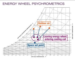
Energy wheels transfer sensible and latent energy. This chart shows how an energy wheel cools and dries outdoor air before it enters the cooling coil, reducing cooling coil requirements. Even without the ASHRAE Standard requirement, energy recovery makes good economic sense. Energy recovery wheels can significantly reduce the mechanical cooling load of a DOAS unit. This reduction of the outdoor air heating and cooling loads will also lead to substantial energy savings.
