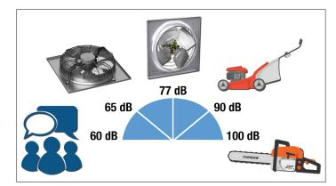
Sound impacts in HVAC equipment can be reduced by selecting components with lower sound features. On average, condenser fans with a swept blade design are up to 12 decibels quieter than traditional paddle fans. There are several component choices that can benefit the unit's acoustic performance, and design choices made by the manufacturer can also impact sound, such as:
